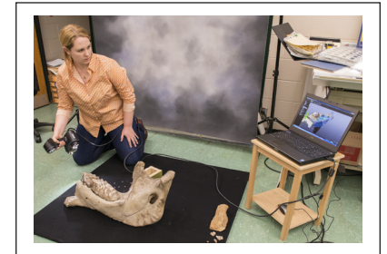
Figure 2: Here, a staff member is 3-D scanning the mastodon jawbone using a Creafom GoScan 50
