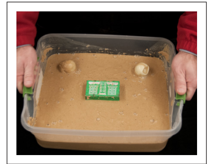
Figure 3: Appearance of the surface area once liquefaction has occurred
